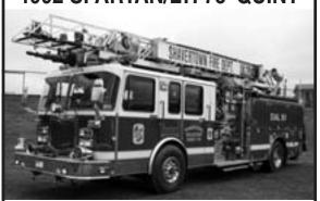
\$110,000.00 OBO Detroit Diesel 8V92 500 HP Allison Automatic transmission rebuilt in July 2013 with 2 year warranty Transmission Retarder (Brake Assist) Approximately 25,000 miles Aerial Hours 695 10 KW Generator 8 Man Spartan Gladiator Cab 5 SCBA seats 300 Gallon Poly Tank 1500 GPM Waterous 2- Stage pump 3-Preconnect Crosslays (2) 1 1/2" and (1) 2 1/2" (1) 2 ½" Discharge Drivers side (1) 5" Intake
